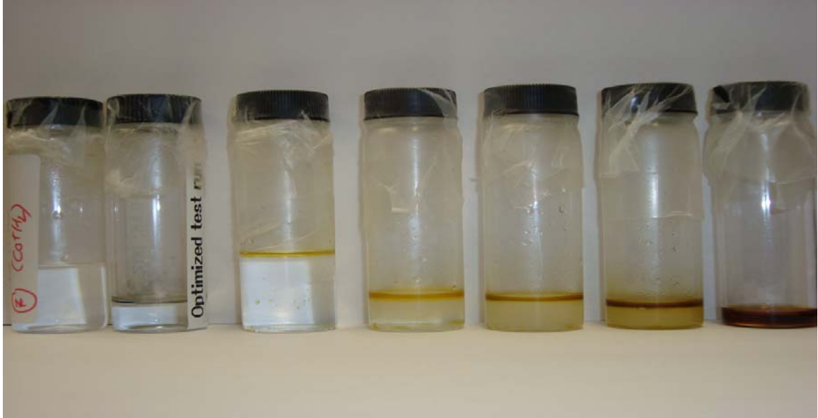
Figure 19. Random samples of FTS liquid product produced from the developed catalysts
